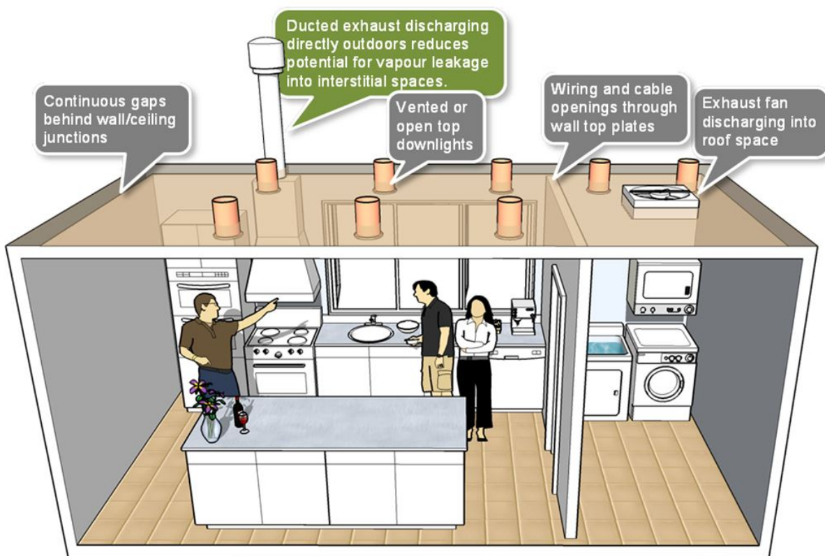
Figure 6.12 Some air and water vapour leakage sites through ceilings
