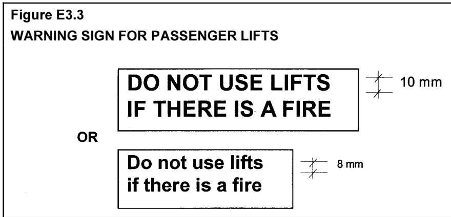
Figure E3.3 WARNING SIGN FOR PASSENGER LIFTS
